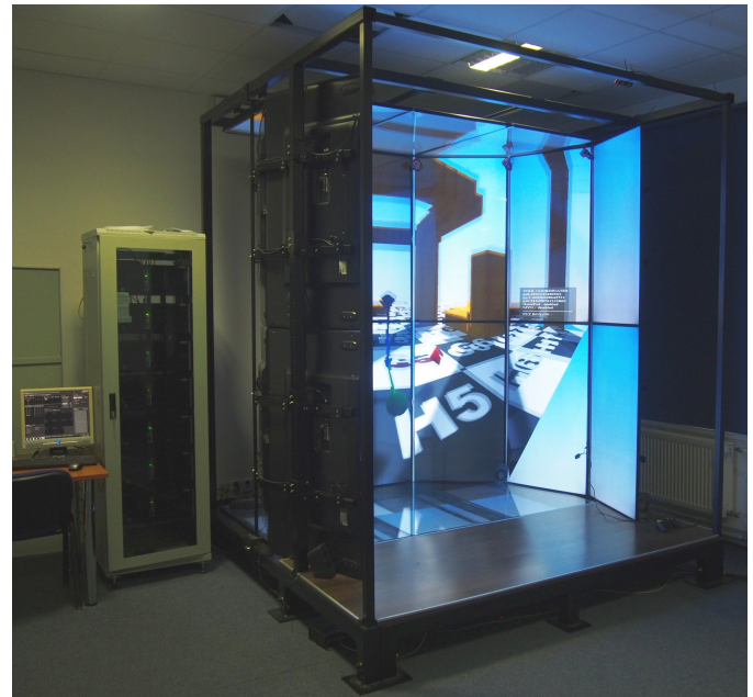
Fig. 1. The LIRKIS CAVE system. From left to right: the LCD display with OptiTrack control software GUI, the computer cluster and the display area.
