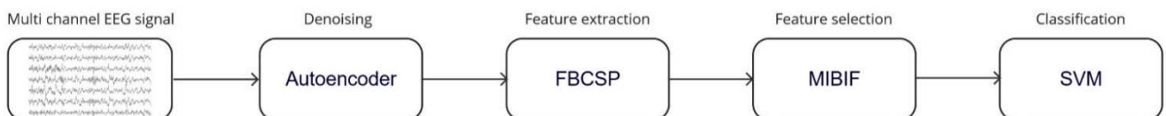
Figure 1: Workflow chart of our proposed algorithm.
